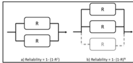
**Figure 3** Reliability in parallel systems (adapted form [11])
