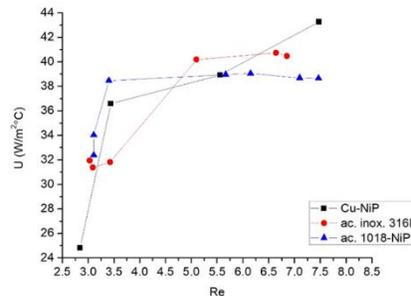
**Graph 5.** Copper and 1018 pipe steel with Ni-P coating against stainless-steel 316L
