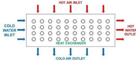
Fig. 1. Diagram of operation of the heat exchanger
