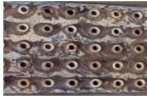
Fig. 2. Exchanger mirror with the presence of corrosion and incrustations
