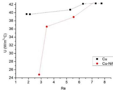
**Graph 2.** Copper pipe under normal state and with Ni-P coating
