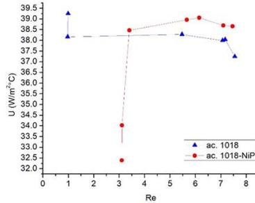
**Graph 4.** Behavior of 1018 pipe steel under normal conditions and with the Ni-P coating
