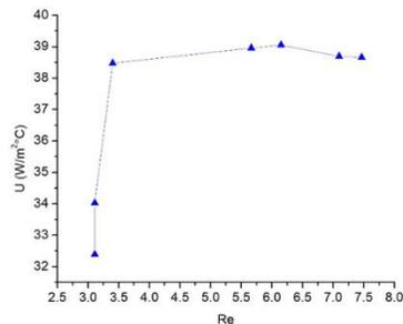
**Graph 3.** 1018 steel pipe with Ni-P coating
