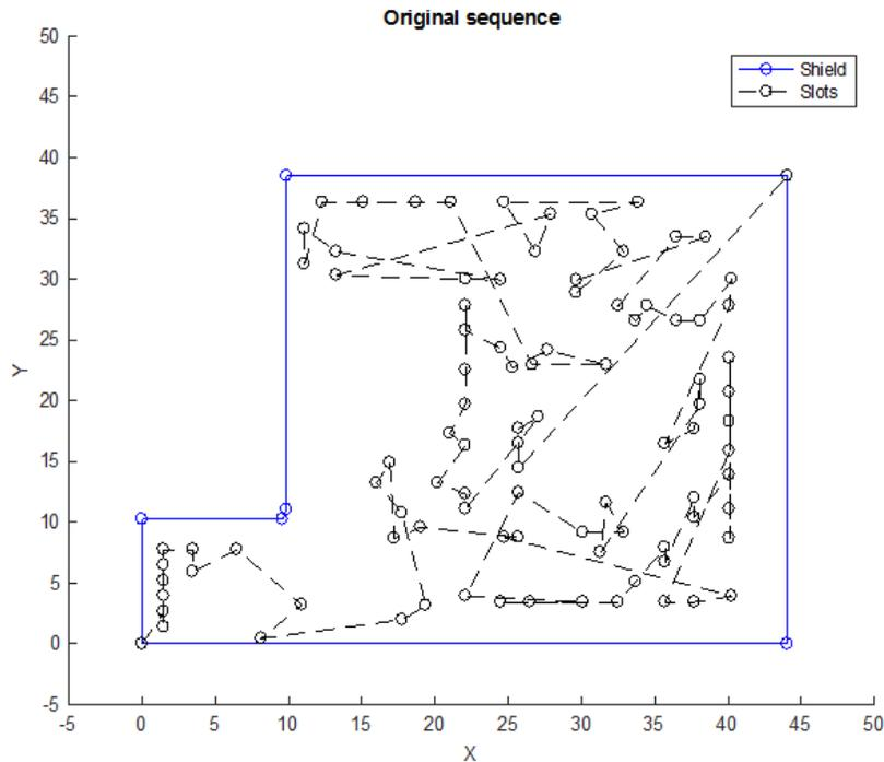
Fig. 7. Original Sequence followed by the printer to print layer 1.
