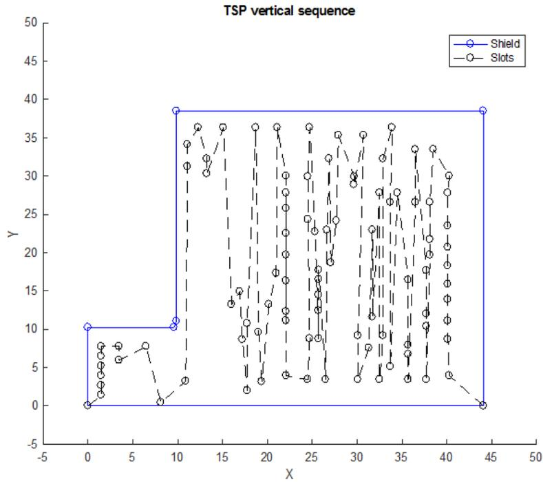
**Fig. 10.** TSP vertical sequence, followed by the extruder to print layer 1.
