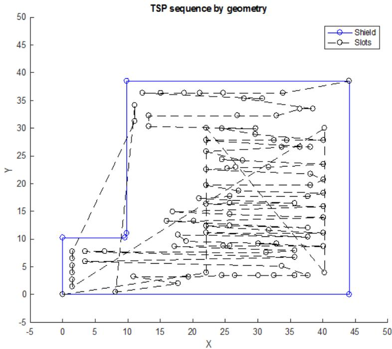
Fig. 8. Sequence by slots geometries, followed by the extruder to print layer 1.
