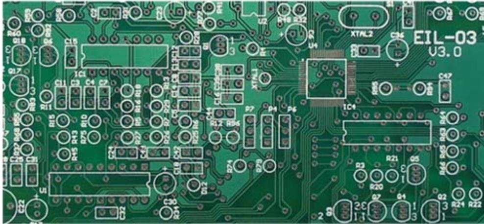
Fig. 3. Part of a PCB of two layers [32].
