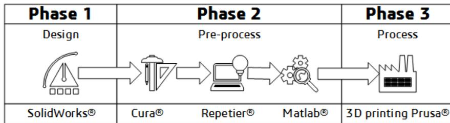
Fig. 4. Method of Optimization of the Fused Filament Fabrication Process in the Manufacturing of Printed Circuit Board.
