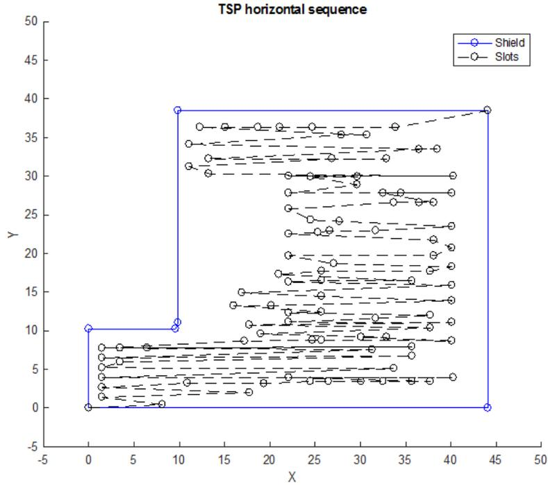
Fig. 9. TSP horizontal sequence, followed by the extruder to print layer 1.
