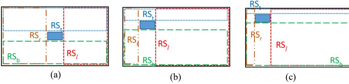
Figure 8: Different residual spaces created by a defect in a plywood sheet.
