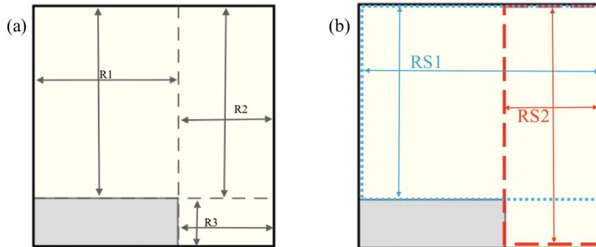
*Figure 1: Definition of a Residual Space*
