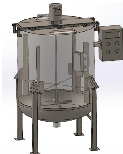
Figure 2. Bottom shaft support in the stirring tank.
